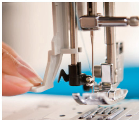
Easy automatic needle threading.
